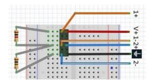
Figure 12: Taking two channels of voltage measurements.
