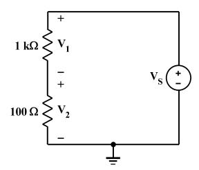
Figure 0: Schematic Diagram of the Voltage Divider.
