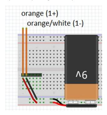
*Figure 8*: *Using header pins to connect Channel 1 to the battery.*
