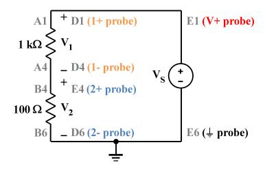
Figure 13: Schematic Diagram of the Voltage Divider.
