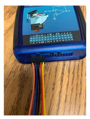
Figure 1: Installing the measurement probes.
